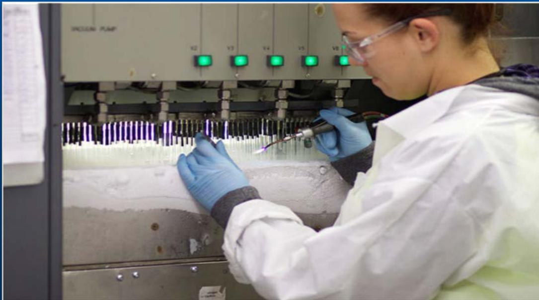
FIGURE F: END-SEALING LIGHT SOURCES
